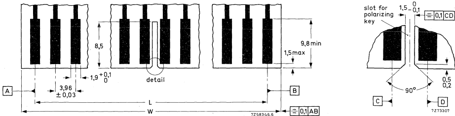
Fig. 4 Recommended dimensions of the printed-wiring board; see Table 4 for dimensions L and W.
